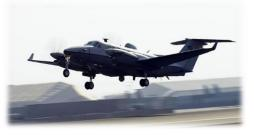
MC-12W – Nine aircraft, along with training, communications, and intelligence support, are based out of Will Rogers IAP, Oklahoma City, OK under the 137th Special Operation Wing (SOW). The 9 aircraft were delivered in the Block 3.1 configuration, to include Extended Range (ER) fuel tanks, day/night full motion video (FMV), Line-of-Sight (LOS) and Beyond-Light-of-Sight (BLOS) video data links (VDL), and digitally
