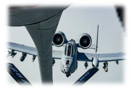
integrated targeting modification, drastically reducing the time required to acquire targets. This ultimately increases both survivability and lethality. ANG A-10 aircraft are equipped with two ARC-210 radios, giving them a unique capability to simultaneously communicate via secure line-of-sight and beyond-line-of-sight, extensively contributing toward successful combat search and rescue missions.
